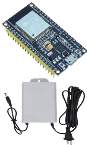
Gambar 2. ESP32 NodeMcu 38pins dan UPS Power Supply
