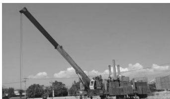
Gambar 2. Hydraulic Static Pile Driver
